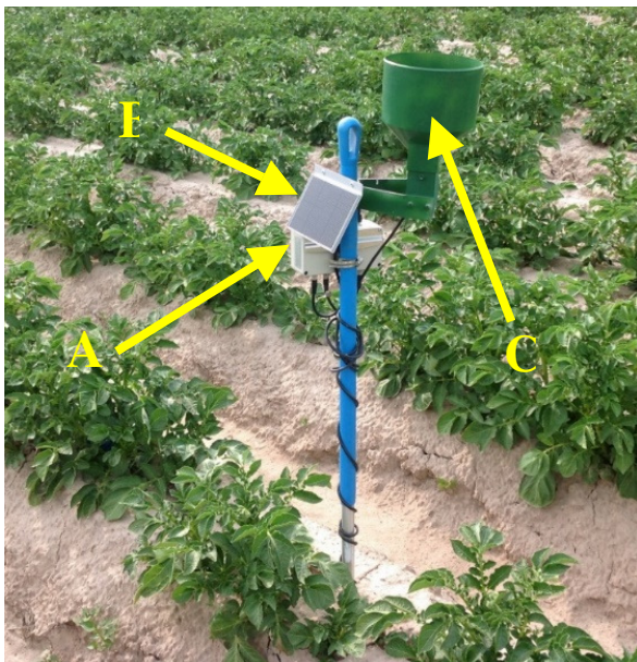
Fig. 4. Measuring complex for recording of rainfall level of precipitation, temperature and water regime of soil state: A – modem; B – solar battery; C – pluviometer; D – probe with humidity and temperature sensors
